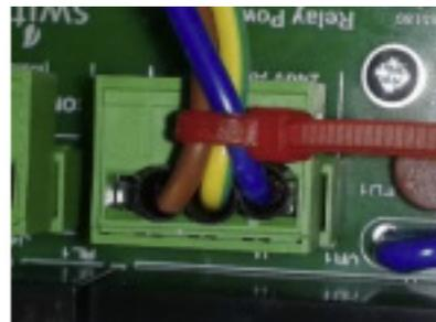
**Important:** If the current boiler control operates at a low voltage, connect the appropriate low voltage to the **COM** (common) and **do not** add the jumper cable.
